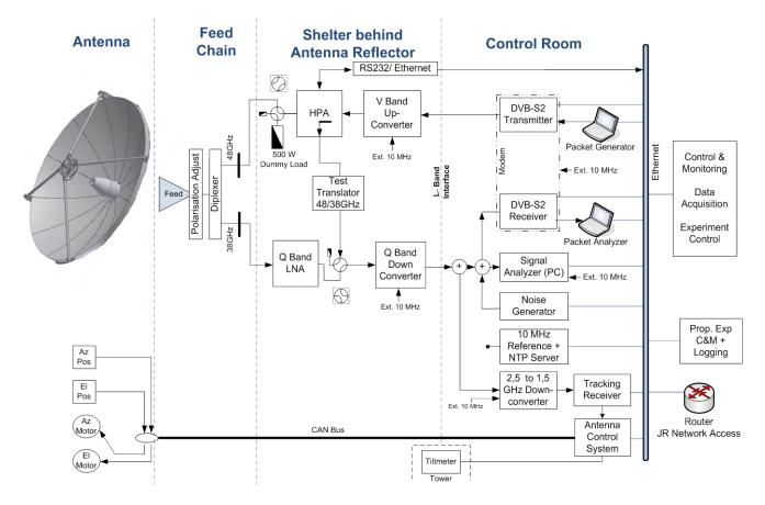
Figure 1: Architectural Design of the Q/V band GS Graz
