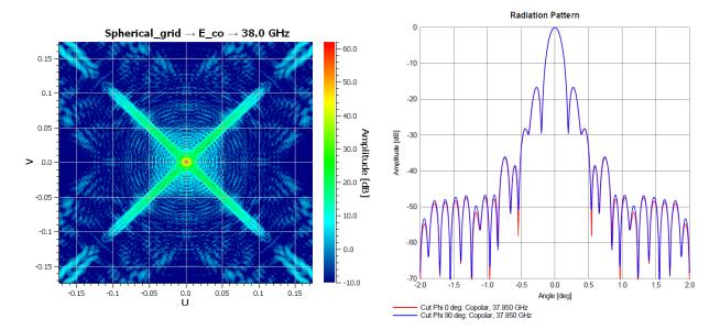
Figure 4: 3D Radiation pattern with struts influence @38GHz and right the RX antenna pattern. © Vertex Antennentechnik
