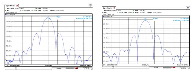
Figure 10: Left: Elevation pattern taken from the Schöckl mountain, 4.06°...6.06°, rate=0.02°/s ; Right: Azimuth pattern taken from the Schöckl mountain, 3.75°... 5.75°, rate=0.02°/s
